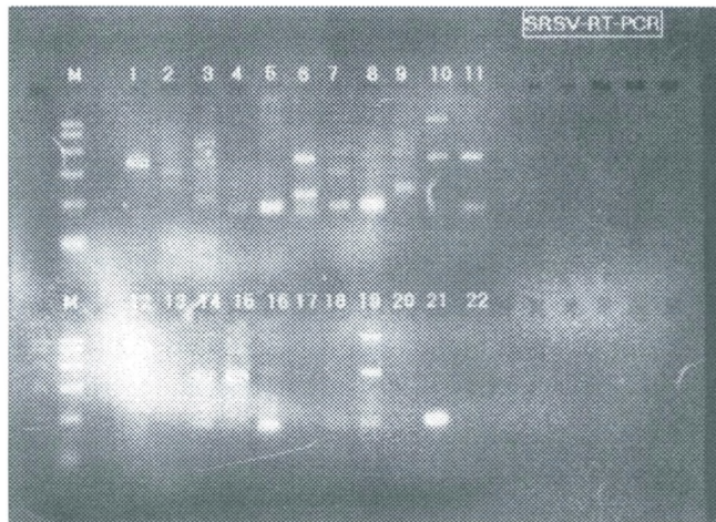
Figure 2. — Electrophoretic separation of PCR-SRSV amplification products in 3% NuSieve agarose gel (containing 0,5 \mu\text{g/ml} ethidium bromide). Positive specimens were number 4, 5, 6, 7, 8, 11, 14, 16, 18 and 19 (clear positive – 5, 7, 8, 11 and 16 while others were mild positive). Clear negative specimens were 12, 13, 17 and 20. All others have had non-specific amplification bands (specimens number 2, 3, 6, 7, 9, 10, 11, 14, 15, 16, 18 and 19). Lane 21 - positive control; lane 22 - negative control (Rnase free destiled water). M – PCR markers: 50, 150, 300, 500, 750 and 1000 bp (Promega Corporation – USA).
